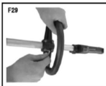
Screw down the bolt and nut (F29)
